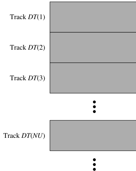
Figure 11.11 Sketch map of unidirectional chained list storage of radar tracks
